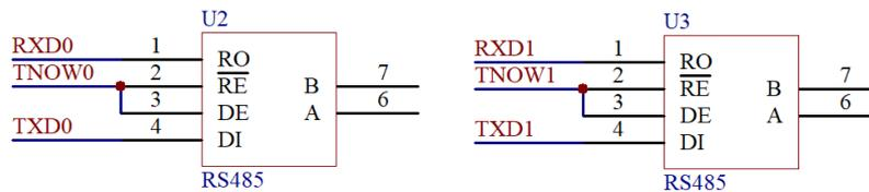
In the figure, TNOW is a switch pin to control the DE (active high transmit enable) and RE# (active low receive enable) pin of RS485 transceiver. The RS485 transceiver should use the same power supply as the VIO.
