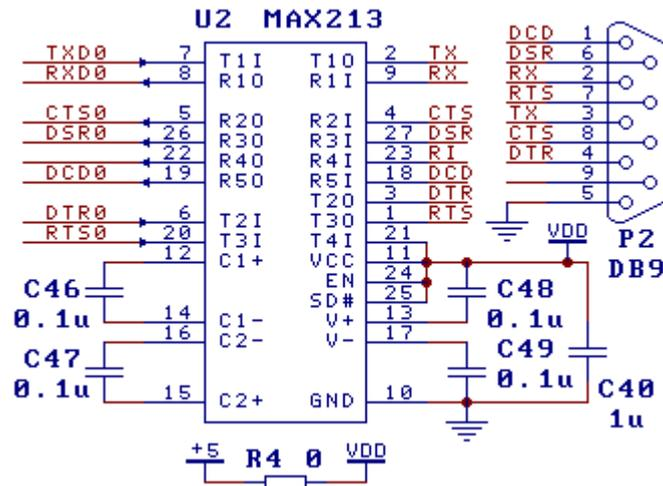
CH9103 provides common UART signals and MODEM signals, the figure shows that one of the TTL UART is converted to RS232 UART by external level conversion circuit U2. The other one is similar with this. Port P2 is DB9 connector, it has the same pins and functions as a normal 9-pin serial port of a computer, chip models similar to U2 include MAX213/ADM213/SP213/MAX211 etc. U2 in the image is uniformly powered by the USB bus through R4.
